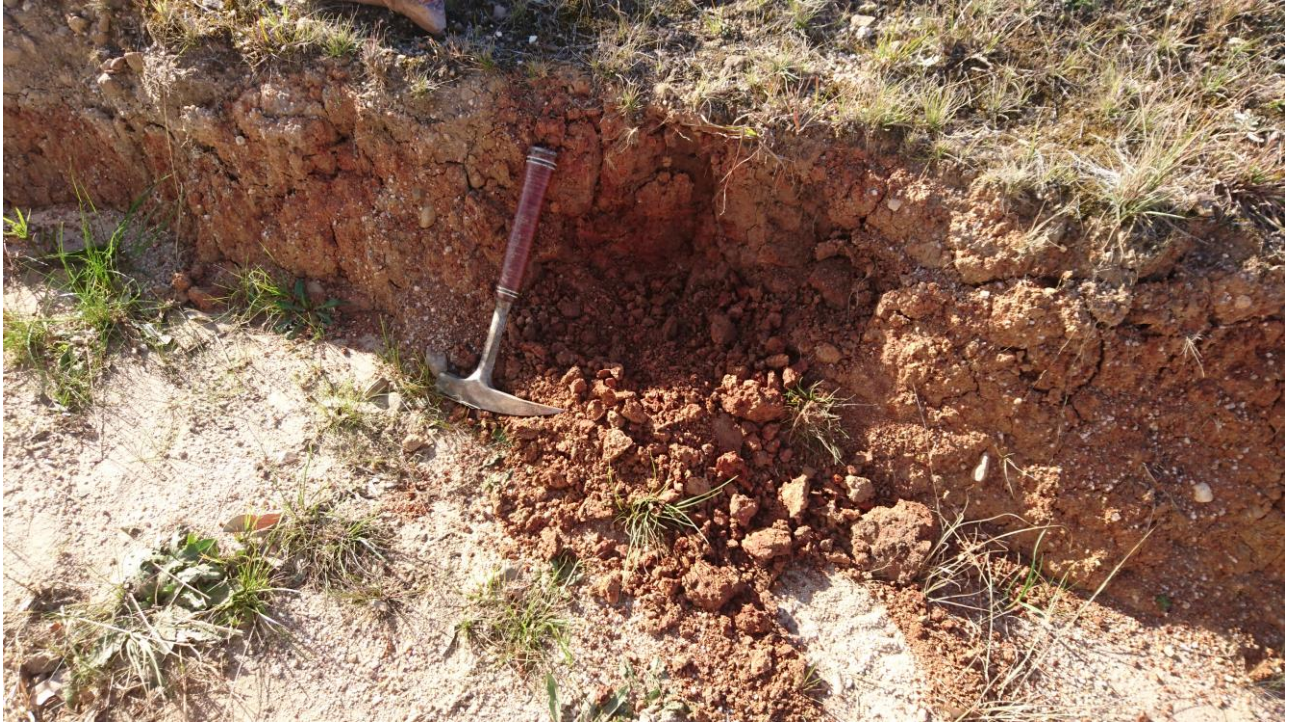
Typical Decomposed Granite Soils
